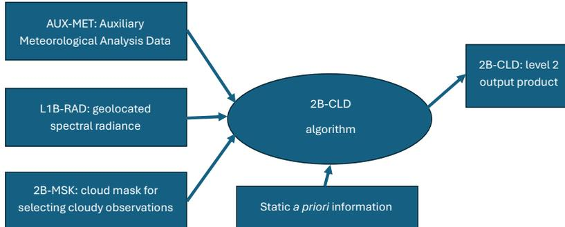
Figure 1.1: Cloud properties algorithm flowchart.
