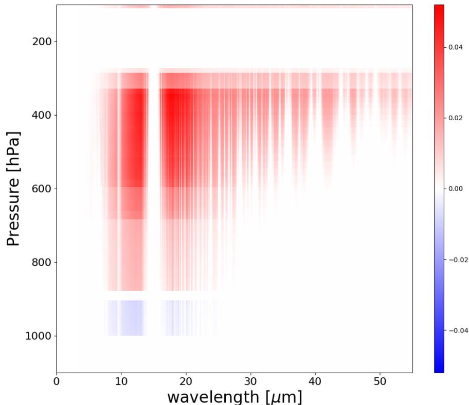
Figure 1.2: Cloud top pressure Jacobian, with units of  $W \text{ (m}^2 \text{ sr } \mu\text{m)}^{-1} \text{ (hPa)}^{-1}$ , at the full PCRTM spectral resolution of  $0.5 \text{ cm}^{-1}$  for a sub-Arctic winter standard profile.
